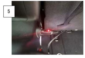
Connect the DC adapter harness plug into the DC outlet located on the driver side interior panel. Installation is now complete.
