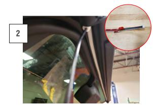
Remove the red tape backing from the LED light strip. Carefully center the LED light strip above the liftgate glass, and apply firm even pressure to the LED light strip to ensure proper adhesion to the liftgate.
