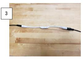
Connect the resistor to the LED light strip, and then connect the opposite side to either the wiring lead, or the DC adapter harness.
