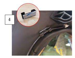
Carefully route the wiring as desired away from any damage that may occur. Secure the wiring using the supplied 3m tape strips, wire holders, and zip ties.
