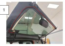
Begin by opening the liftgate. Using isopropyl alcohol, clean around the top of the glass, and down the side where the LED Light strip will be installed. Allow time to dry. Use the red dotted lines above as a reference.
