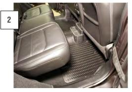
Rear floor mat is one piece. Begin by inserting one side at time. Secure the floor mat to the factory floor locators. Installation is now complete.
