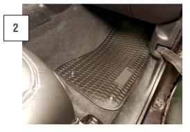
Insert the new floor mat, and secure to the factory floor locators. Repeat on the opposite side.
