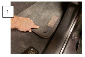
Begin by pulling up to release the factory floor mat from the locators. Remove floor mat. Vacuum any debris. Repeat on the opposite side.
