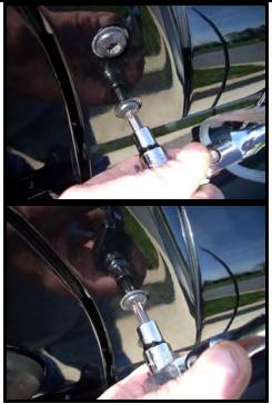
Step 3: Remove the front 2 torx head bolts from the windshield retainer bracket. (DO NOT DISCARD THESE BOLTS Both these bolts will be
