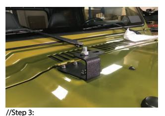
Once mounts are secured, install the (2) M12x1.75 30mm bolts through the bottom of the bracket with (2) M12x1.75 Locking Nuts per side.
