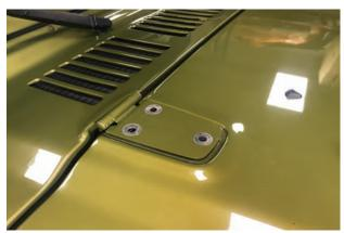
**// Step 1:** Remove the (3) T40 Torx bolts from the hood hinge.
