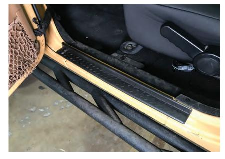
//Step 3: Press door sill on to vehicle firmly. Apply firm even pressure to ensure proper adhesion.
