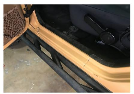
//Step 1: Clean vehicles surface with a alcohol cleaning pad to give the double sided tape a good surface to stick to.
