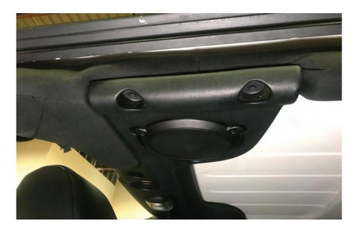
//Step 1: Remove (2) 10mm bolts partially securing the speaker to the roll bar.
