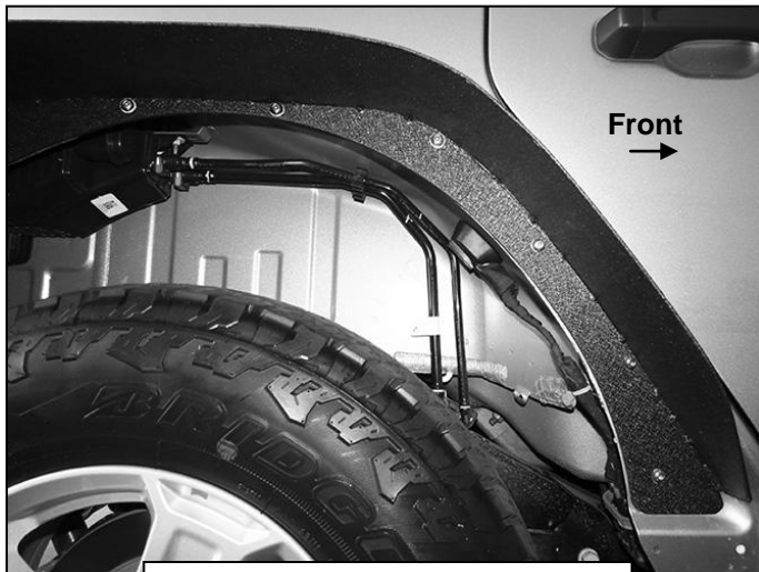
(Fig 12) Attach front of Fender to mounting locations on body
