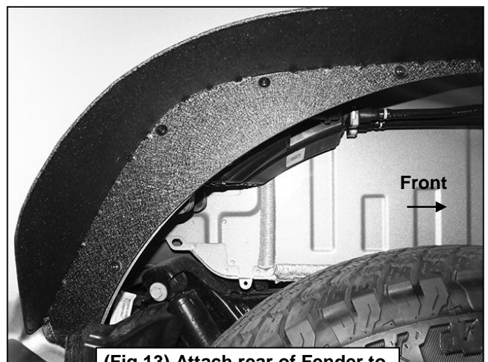
(Fig 13) Attach rear of Fender to mounting locations on body
