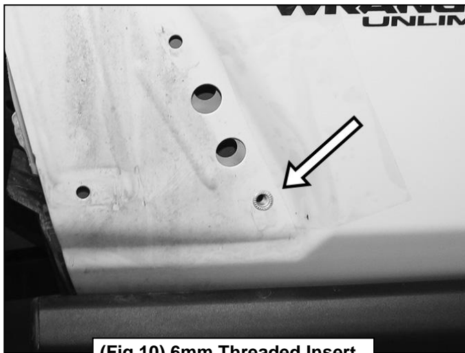
(Fig 10) 6mm Threaded Insert fully installed (arrow)
