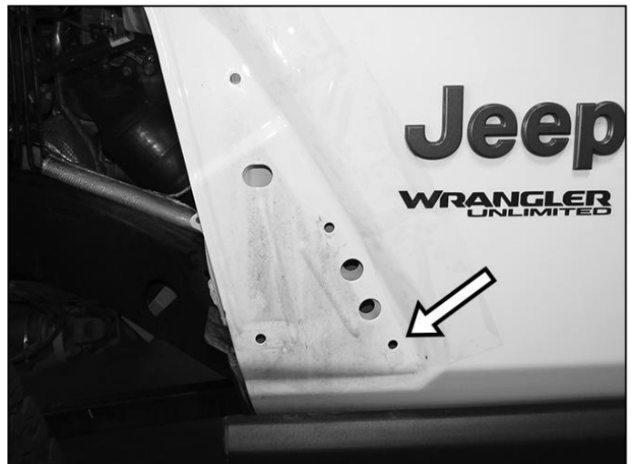
(Fig 8) Use a 25/64" drill bit to open hole up slightly for Threaded Insert installation (see Fig 7)
