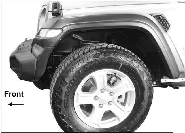
(Fig 1) Release clips attaching fender liner to outer fender
