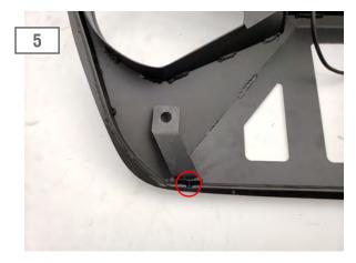
Install the lower grille brackets to the grille using the (2) M6x1.0x20mm bolts, flat washers, and nuts. \*\*Note: Do not fully tighten hardware. Leaving hardware loose, will allow ease of installation in a later step.
