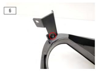
Install the upper grille brackets to the grille using the (2) M6x1.0x20mm bolts, flat washers, and nuts. \*\*Note: Do not fully tighten hardware. Leaving hardware loose, will allow ease of installation in a later step.
