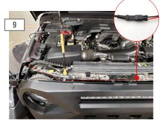
Starting from the battery, route the supplied harness connector along the fender, radiator support and to the LED light bar. Connect the supplied harness connector into the LED Light bar. Zip tie any excess wire away from moving and/or hot engine components.
