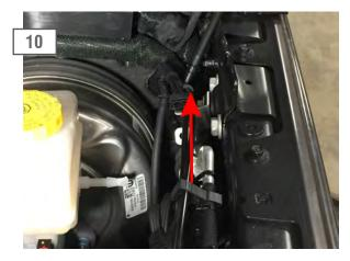
Route the on/off switch to the interior of the vehicle through a suitible body grommet. Mount the switch in the desired location. Zip tie any extra loose wiring out of the way.
