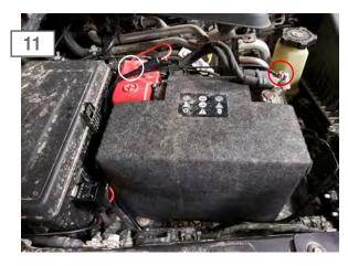
Install the Red 12v + wire to the positive battery terminal. Connect the Black - ground wire to the negative battery terminal. Mount the relay switch in desired location.
