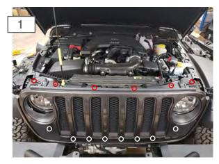
Begin by removing the (6) upper push pins using a trim panel removal tool. Carefully pry the grille away from the vehicle, and remove the grille. \*\*Note: White circles indicate locations of the metal retaining clips to pry away from vehicle to remove grille.
