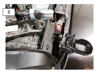
Attach the upper grille bracket to the upper radiator support using the hardware from Step 3. Center the grille side to side. Once grille is centered, fully tighen the upper and lower grille brackets to the grille from Steps 5 & 6.
