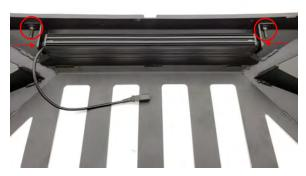
Install the LED light bar brackets to the grille using the (2) M8x1.25x40mm bolts, flat washers, and lock nuts. Then install the LED light bar to the brackets using the (2) M8x1.25x15mm bolts, lock washers, and flat washers.
