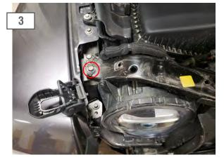
Locate, and remove the (2) 13mm bolts from the upper radiator support. \*\*Note: These bolts will be reused in a later step.
