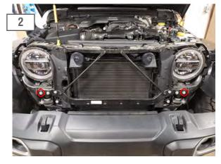
Locate, and remove the (2) 13mm bolts from the lower radiator support. \*\*Note: These bolts will be reused in a later step.
