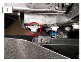
Attach the lower grille bracket to the lower radiator support using the hardware from Step 2. \*\*Note: It is best to use a 13mm wrench to tighten because the lack of space between the grille and the bolt.
