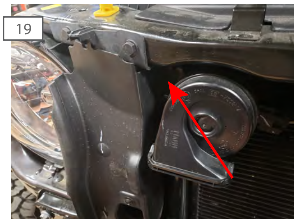
Feed the LED light bar wiring through the radiator support. Plug the light into the light bar harness, and ensure the plugs clip together.
