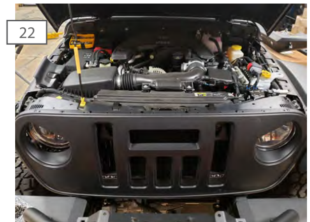
Temporarily install the grille. Adjust the LED light bar as desired. Remove the grille to tighten the LED bolts. Carefully press in the lower portion of the grille until it clicks in place. Then secure the upper portion using the factory (6) push clips. Installation is now complete.
