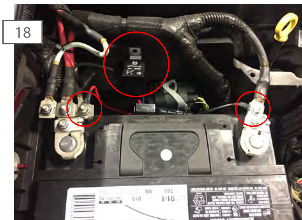
Connect the Red ring terminal to the positive (+) battery terminal. Connect the Black ring terminal to the negative (-) battery terminal. Secure the relay out of the way.
