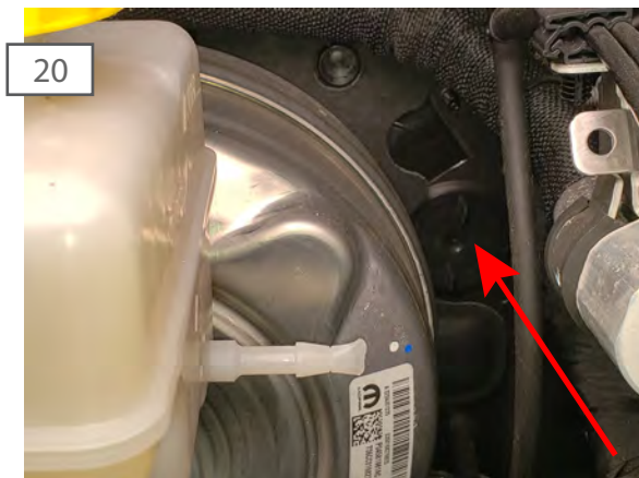
Feed the switch wiring through a firewall grommet into the interior of the vehicle. Mount the switch as desired.
