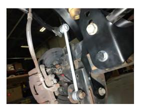
Install the track bar bracket by removing the lower control arm bolt. Slide the bracket over the factory bracket. Install the lower control arm bolt. Loosely install the U-bolt on the axle. Then install the supplied 14mm bolt and spacer into the factory bolt location. Use the factory bolt and flange nut to mount the track are in the lowest hole.
