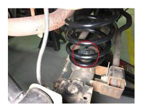
Install the brake line relocation brackets using the 1/4" x 1" bolt, washer, and lock nut.
