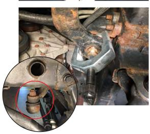
Re-install the supplied pitman arm reusing the factory lock washer and nut. Re-install the tie rod bar.
