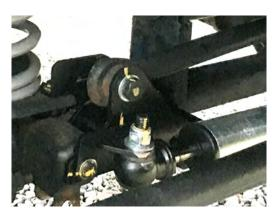
Start by placing the track bar relocation bracket on the factory mount. Install the factory track bar bolt, install the supplied crush sleeve on the factory bolt.
