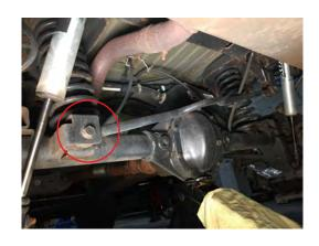
Remove the bolts holding the brake lines to the frame to allow for slack when lowering the axle.
