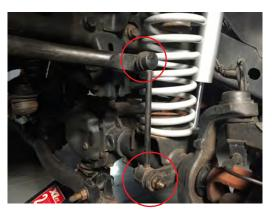
Using the supplied brake line relocation brackets and 1/4" x 1" bolts, washers, and nuts, relocate the factory brake lines. \*\*Note: Gently massage the factory brake line ensuring they do not get kinked. It is important to make sure the brake lines don't make contact with anything, this can cause the brake lines to rub through causing you to lose your brakes.
