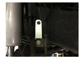
Reinstall the shocks, and track bar. Double check all bolts are installed and torqued to factory specifications prior to reinstall the front wheels and lower the vehicle.
