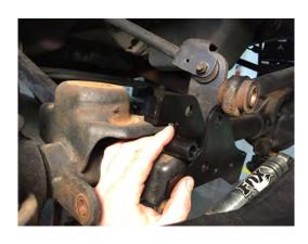
Install the supplied U-bolt, washers, and nuts around the axle and through the track bracket.
