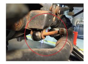
Install the track bar relocation bracket. \*\*Note: If reusing the stabilizer shock install the stabilizer shock relocation bracket with the track bar relocation bracket. See picture.
