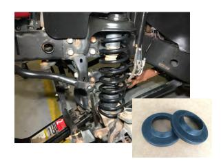
Remove the factory stabilizer and bracket from the axle mount.
