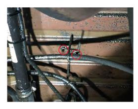
Remove the rear sway bar end link. This end link will be reused on the front sway bar.
