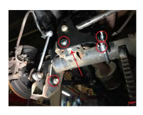
Reinstall the shocks. Double check all bolts are installed and torqued to factory specifications.
