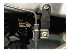
Install the supplied bump stops using the supplied 5/16x1.25" bolts.
