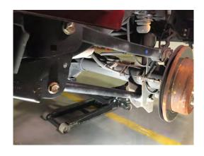
Lower the rear axle slowly and remove the rear springs. Retain the upper rubber spring isolator for use with the new spring.
