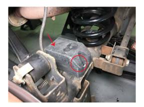
Install the supplied sway bar end-link using the factory lower nut and bolt.
