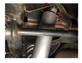
Remove the ABS wiring clip from the axle to allow more slack when lowering the axle.
