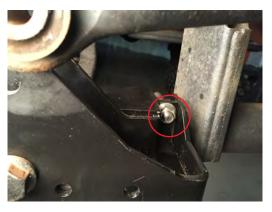
Using the supplied 3/8"x 1 1/4" bolts, washers, and nuts, mount the stabilizer shock relocation bracket through factory pre drilled holes.
