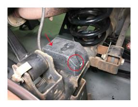
Install the supplied sway bar end-link using the factory lower nut and bolt.
