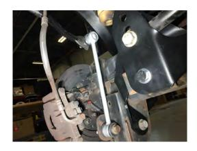
Install the track bar bracket by removing the lower control arm bolt. Slide the bracket over the factory bracket. Install the lower control arm bolt. Loosely install the U-bolt on the axle. Then install the supplied 1/2" bolt and spacer into the factory bolt location. Use the factory bolt and flange nut to mount the track bar in the lowest hole. Tighten the U-bolt before moving to the next step.
