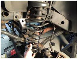
Center the supplied bump stop extension on the spring perch. Using a marker, scribe the hole location. Remove the extension and drill the hole location to 3/8".
