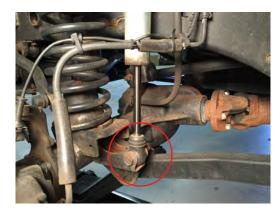
Remove the brake line bracket, this will allow you to lower the axle to remove the factory spring.
