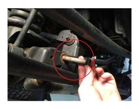
Remove the sway bar end links from the axle and the sway bar. The link will not reused, but the hardware will be.
