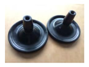
Install the supplied rear springs(short Spring), Be sure to reuse the upper rubber spring isolator. Install the rear spring retainers (Large Washers) using the supplied 3/8"x1" bolt with lock washer and flange nut.
