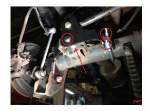
Reinstall the shocks. Double check all bolts are installed and torqued to factory specifications.
