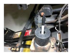
Place the bump stop extension loosely in the supplied front spring(Long Spring). Do not try to bolt the extension down prior to installing the spring. With the bump stop in the spring install the spring into the factory location using spring spacer and factory isolator. Position the bump stop over the pre-drilled hole and secure using the 3/8" x1.25" bolt, washers, lock washer, and nut. Ensure the
