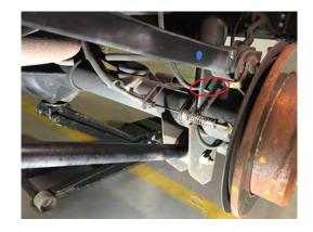
Remove the 10mm nuts holding the brake cables to the body of the vehicle.
