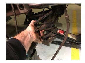
Install the supplied upper spring spacer. Use a silicone based lubricant and press the spacer into the factory location.
