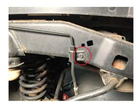
Remove the factory shocks from the axle and the upper mount. The factory hardware will be reused.
