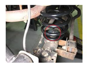
Remove the factory brake lines from the chassis and brake caliper. Install the supplied brackets using the factory hardware and supplied retaining clip. Reconnect the brake line to the caliper using the supplied crush washers. Always bleed the brakes prior to lowering the vehicle from the jack stands.
