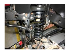
Remove the factory rear sway-bar end links, reinstall them on the front using the factory hardware. The swivel end mounts to the way bar, the other end mounts to the axle using factory hardware.
