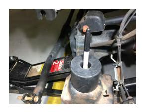
Place the bump stop extension loosely in the supplied front spring(Long Spring). Do not try to bolt the extension down prior to installing the spring. With the bump stop in the spring install the spring into the factory location using the factory isolator. Position the bump stop over the pre-drilled hole and secure using the 3/8" x1.25" bolt, washers, lock washer, and nut. Ensure the
