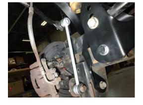
Install the track bar bracket by removing the lower control arm bolt. Slide the bracket over the factory bracket. Install the lower control arm bolt. Loosely install the U-bolt on the axle. Then install the supplied 14mm bolt and spacer into the factory bolt location. Use the factory bolt and flange nut to mount the track bar in the lowest hole.
