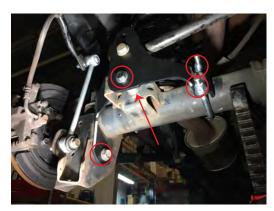
Reinstall the shocks. Double check all bolts are installed and torqued to factory specifications. \*\*Prior to tightening the lower control arm bolts, reinstall the wheels and tires. Lower the vehicle off the jack stands. With the vehicle at ride height, torque the lower control arm bolts to 125 ft/lbs.
