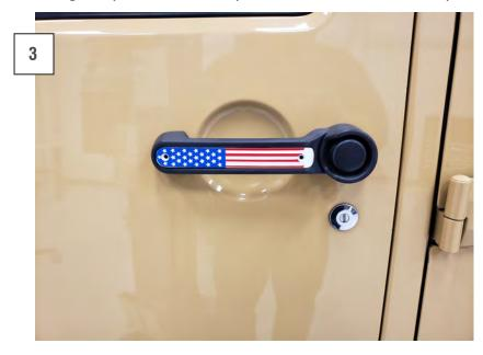
Secure the door handle insert with (2) of the supplied screws. Repeat this process for the remaining door handles, and rear tailgate handle. Installation is now complete.
