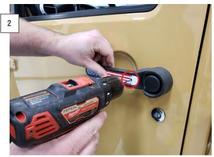
Position the door handle insert in place, and carefully drill the (2) 1/4" holes into the factory door handle. \*\*Note: Do not drill all the way through. Only drill into the factory door handle about 1/4" of the way.
