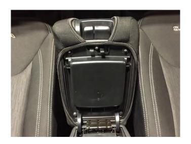
**Step 3\\**Complete the installation by stretching the cover over the arm rest and wrapping it around the back edge of the arm rest.
