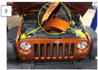
Using a soft pry tool, remove the (2) plastic push clips, (1) on either side of the grille. These will be reused to attach the Brow. Test fit the Brow before removing the tape backing.
