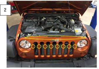
Thoroughly clean the grille cover with soap and water to remove any dirt, oil, grease, wax, etc. \*\* Recommended: Use isopropyl alcohol to wipe the painted surfaces that will make contact with the 3M tape. A clean surface is essential for proper adhesion of the 3M tape. Allow the grille surface time to thoroughly dry before continuing to Step 3.
