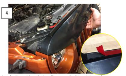
Once familiar with how the Brow fits, remove the (8) small pieces of tape and fold back only a corner of the strip that runs along the top edge. Hold the bottom of the Brow off the grille while you install the factory push clips, then pull off the folded back portion of the tape backing. Push the bottom of the Brow against the grille seating the (8) small pieces of tape to the vehicle. Apply firm even pressure to all taped surfaces to ensure proper adhesion.
