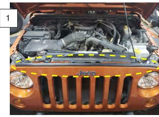
Open and support the hood. Locate the factory weather stripping. Using a soft tool, pry the weatherstripping off the factory grille. Factory weatherstripping will not be reused. \*\*Note: If there is any remaining adhesive on the paint. A quality adhesive remover will need to be used to remove the remaining adhesive.
