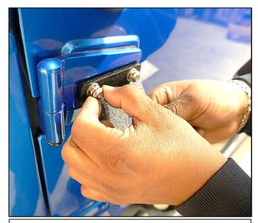
Step 2. Place a supplied M8x1.25x30mm button head bolt (F) with supplied M8 flat washer (G) and supplied M8 split washer (H) through the hole in the bracket through the hole in the door hinge onto factory hood. Repeat step for remaining bolt. Once all hardware is installed tighten down all hardware. Repeat step 1-3 for remaining bracket.
