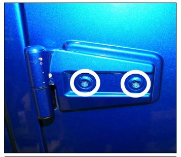
Using a T-50 torx bit locate and remove two factory bolts on the door hinge. Discard factory hardware.
