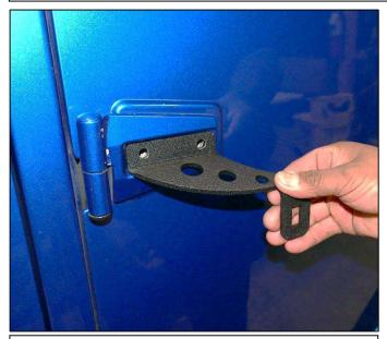
Step 1. Place supplied mounting bracket (A) onto Jeep. Line up the bracket holes with the holes in the door hinge holes.
