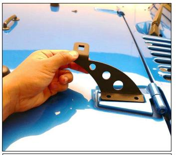
Step 2. Place supplied mounting bracket (A) onto Jeep. Line up the bracket holes with the holes in the hood hinge holes.
