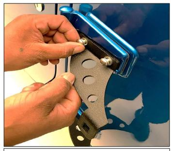
Step 2. Place a supplied M8x1.25x30mm button head bolt with supplied M8 flat washer (G) and supplied M8 split washer (H) through the hole in the bracket through the hole in the door hinge onto factory hood. Repeat step for remaining bolt. Once all hardware is installed tighten down all hardware. Repeat step 1-3 for remaining bracket.
