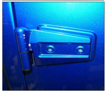
Step 1. Using a T-50 torx bit locate and remove two factory bolts on the door hinge. Discard factory hardware.
