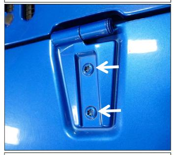
Step 1. Using a T-50 torx bit locate and remove two factory bolts on the hood. Discard factory hardware.
