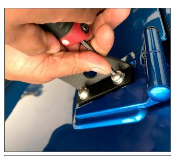
Step 3. Place a supplied M8x1.25x30mm button head bolt with supplied M8 flat washer (G) and supplied M8 split washer (H) through the hole in the bracket through the hole in the hood hinge onto factory hood. Repeat step for remaining bolt. Once all hardware is installed tighten down all hardware. Repeat step 1-3 for remaining bracket.
