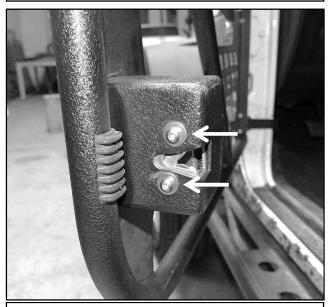
Step 2. Using a 5/32 allen wrench loosen up two allen head bolts holding the door latch onto door.
