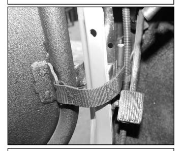
Step 2. Attach the new door stopper strap onto vehicle.
