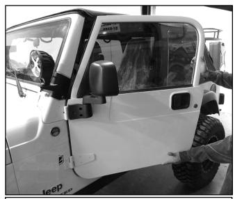
Step 3. Lift the door off the hinges. Set factory door aside in a protected area. Repeat step 1-3 for other side of vehicle.
