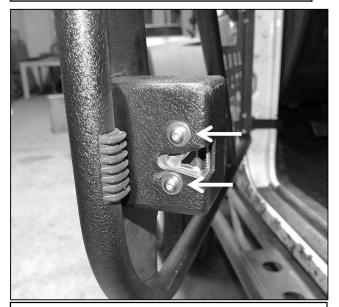
Step 2. Using a 5/32 allen wrench loosen up two allen head bolts holding the door latch onto door.
