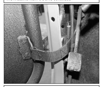
Step 2. Attach the new door stopper strap onto vehicle.
