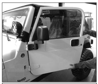
Step 3. Lift the door off the hinges. Set factory aside in a protected area. Repeat step 1-3 for other side of vehicle.
