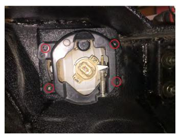
**Step 2\\**Locate the (4) factory screws, and remove. \*\*Note: Factory hardware will be reused.
