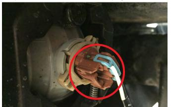
**Step 1\\**Access the connectors on the rear of the fog lights from the wheel well, and remove. \*\*Note: Light connector will be different between 07-09 and 10-18.
