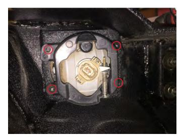
**Step 2\\** Locate the (4) factory screws, and remove. \*\*Note: Factory hardware will be reused.
