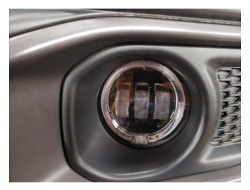
**Step 4**\\ Plug the supplied wiring connector harnesses into each factory fog light connector and then connect to the new fog lights. Installation is now complete.
