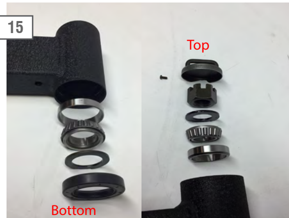
15 Install the larger bearing and race into the bottom of the tire carrier, and the smaller bearing and race on the top of the tire carrier. Make sure to pack the bearing with grease before installation. Then use the small washer for the top and the larger washer for the bottom. Install the seal on the bottom of the tire carrier. Also use a small amount of grease for the seal.
