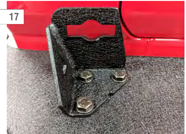
17 Install the latch bracket to the rear bumper by using the (3) M10 x 40mm bolts, (6) flat washers, and (3) lock nuts.
