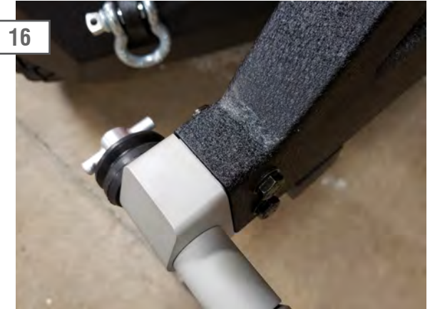
16 Install the latch to the carrier arm by using (2) M10 x 65mm bolts, (4) flat washers, and (2) M10 lock nuts.
