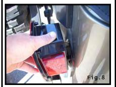
Step 5: Carefully guide the wiring back through the hole and reinstall the tail lamp using the factory hardware. Becareful not to over tighten.
