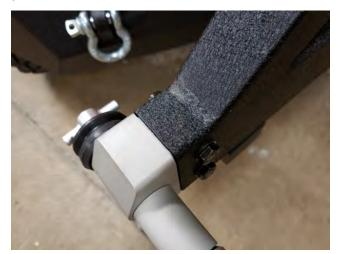
**STEP 16 //** Install the latch to the carrier arm by using (2) M10 x 65mm bolts, (4) flat washers, and (2) M10 lock nuts.
