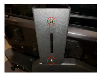
**STEP 21 //** IInstall the upper bracket to the lower bracket using the (2) M6x1.0x25mm bolts, flat washers, and lock nuts.
