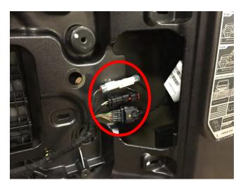
**STEP 12 //** Locate, and unplug the (3) wire connections.
