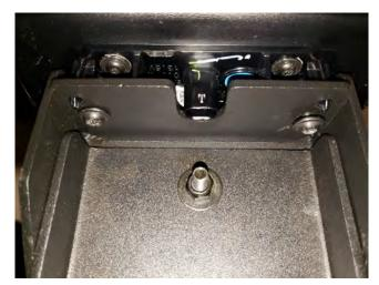
**STEP 22 //** Remove the screws holding the 3rd brake light to the factory tire carrier. Transfer the 3rd brake light to the new bracket. Carefully tighten the factory torx screws. The screw bosses are plastic and can strip out easily. **J130318-JL**
