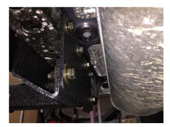
**STEP 10 //** Install the hitch assembly and hitch plate using the (4) M12x120mm bolts, and (2) M12x40mm bolts, flat washers, and lock washers. Torque to 40 ft-lbs. **J130318-JL**
