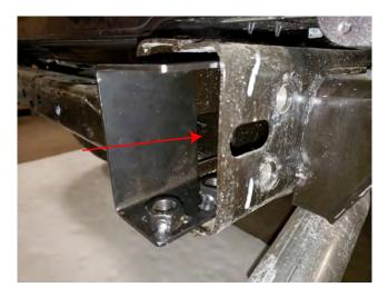
**STEP 7 //** Insert the supplied dual nut plate into the passenger side frame rail.
