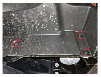
**STEP 4 //** Locate and remove the (3) 8mm screws securing the splash shield to the bumper. Remove splash shield.
