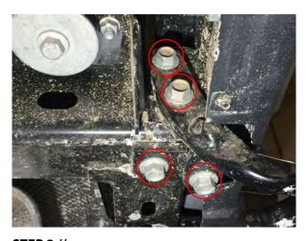
**STEP 2 //** Locate and remove the (4) 21mm bolts securing the tow hook. Remove tow hook.
