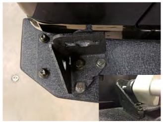
**STEP 17 //** Install the latch bracket to the rear bumper by using the (3) M10 x 40mm bolts, (6) flat washers, and (3) lock nuts.
