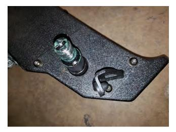
**STEP 14 //** Install the bumper plate using the (3) M6x1.0x10mm bolts, flat washers, and lock washers.
