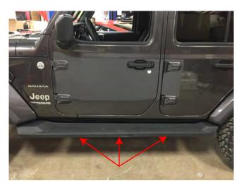
**STEP 1 //** Begin by locating the (3) pinch weld mounting locations under the vehicle.
