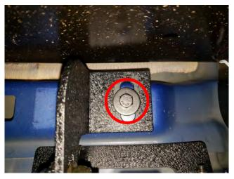
**STEP 5 //**Position the new Rocker Step and install them by using the (2) M8x35mm bolts, flat washers, and lock washers through the body mount brackets. \*\*Note do not fully tighten leaving room for some adjustment.
