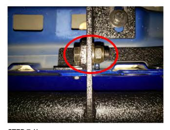
**STEP 7 //**Connect the pinch weld brackets to the Rocker Step body mount brackets by using the (2) M10x35mm bolts, flat washers, and lock nuts. Next fully tighten the body mount brackets from Step 5. \*\*Note If front to back adjustment is needed, loosen the hardware from Steps 5 & 7 to achive the position desired then re-tighten fully.
