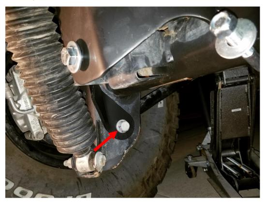
7. Next, fully tighten and torque all 3 mounting points. Torque the U-bolt to 45ft/lbs, the control arm bolt to 125ft/lbs, and the supplied center bracket bolt to 75ft/lbs.
