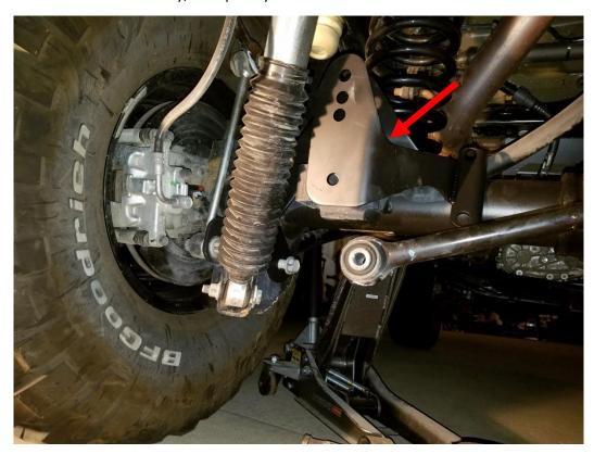
**4.** Using the supplied hardware, attach the new bracket to the factory track bar mount. Insert the supplied bolt and washer though the bracket, then through the spacer sleeve where the track bar was originally mounted. Then loosely tighten the nut using a ¾" wrench and ¾" socket.
