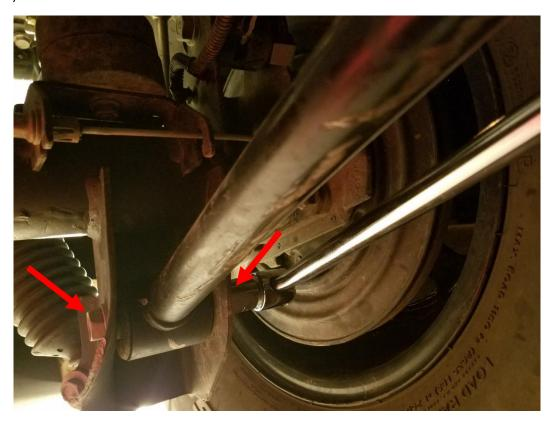
2. Use a 21mm socket and breaker bar, remove the track bar bolt and flag nut.
