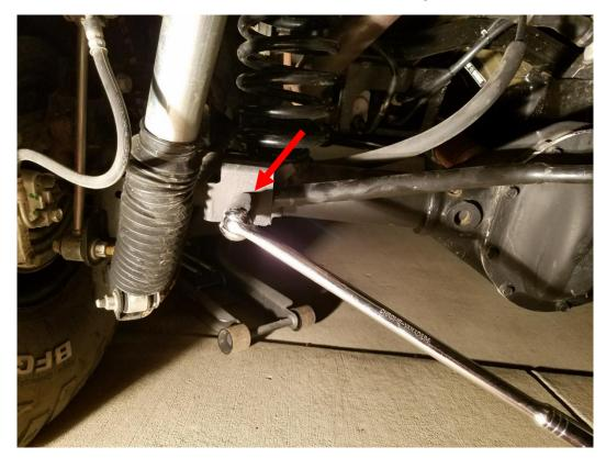
3. Lower the track bar out of the way, then place your new trackbar bracket over the stock track bar mount.
