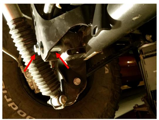
5. Install the supplied U-bolt, washers and nuts as shown. Using a ¾" deep well socket, loosely tighten the nuts.
