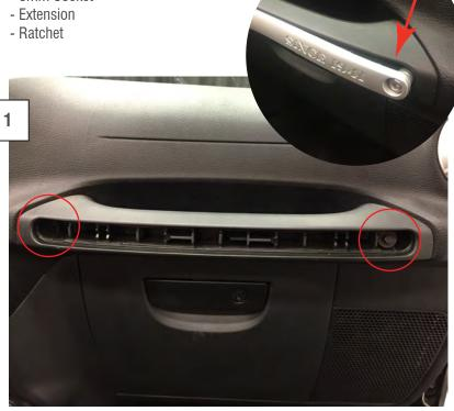
Begin be removing the trim panel from the grab handle. Use a soft pry tool to remove the panel from the dash. Next, remove the (2) 8mm bolts securing the handle to the dash.
