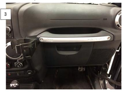
Reinstall the grab handle using the factory 8mm screws. Reinstall the factory trim panel.
