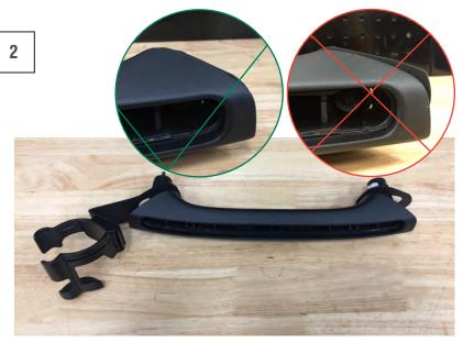
Place the spacer over the passenger side of the grab handle. Note if the spacer doesn't fit well, flip it over. Place the phone/cup holder over the driver side of the grab handle.
