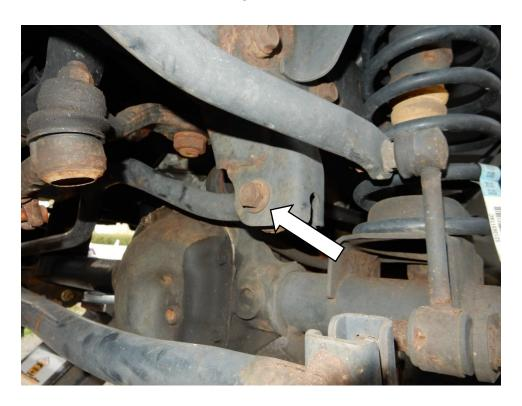
2. Using a 21mm socket, remove the bolt connecting the front track bar to the axle bracket. Remove the front track bar.
