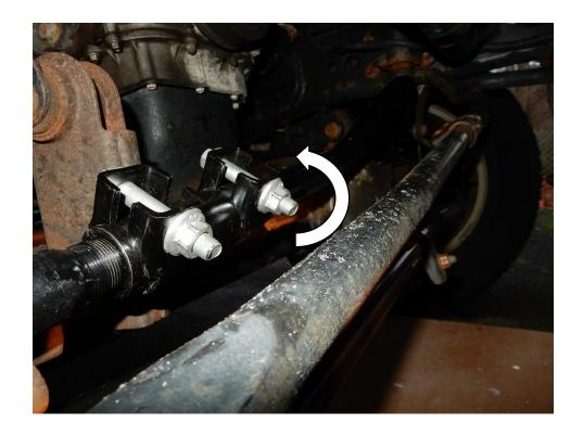
8. Using a 15mm socket, tighten the bolts on the adjustment sleeve. Torque to 45 ft-lbs.
