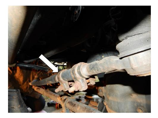
11. Using a 15mm socket, loosen the nuts on the adjuster sleeve of the drag link. Rotate the adjuster sleeve of the drag link clockwise approximately 3/4 of a turn or as needed until the steering wheel is straight.
