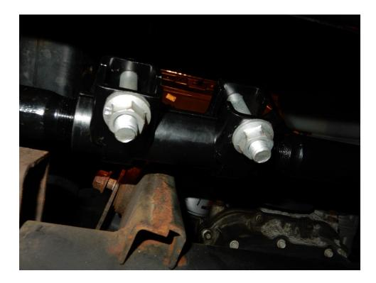
7. Rotate the track bar adjustment sleeve clockwise until the dimensions noted from step 5 are the same on both the driver and passenger sides.
