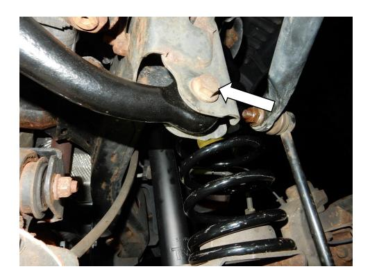
4. Using a 21mm socket, install the track bar into the axle side bracket using the factory bolt and nut. Torque to 125 ft-lbs.
