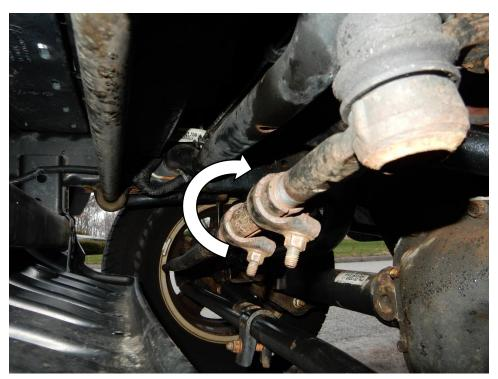
12. Using a 15mm socket tighten the nuts on the adjuster sleeve of the drag link. Torque to 45 ft-lbs.
