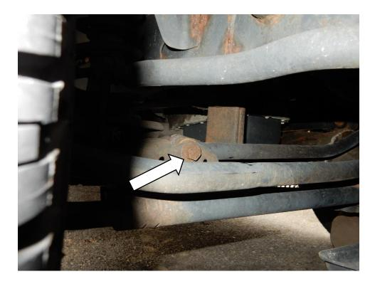
3. Using a 21mm socket and wrench, install the track bar into the frame side bracket using the factory bolt and nut. Torque bolt to 125 ft-lbs.
