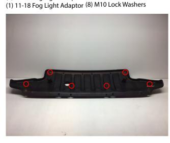
**STEP 1** // Remove the (6) plastic push pins securing the factory splash shield to the vehicle. (4) Across the front edge, (2) on the rear edge.
