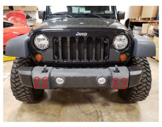
**STEP 3** // From under the vehicle, access and remove the (8) 18mm nuts securing the factory bumper to the vehicle.
