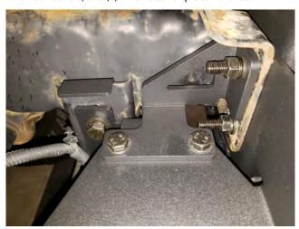
**STEP 9** // Secure the (2) winch plate brackets to the winch using the (4) M10x1.5x50mm bolts, (4) lock washers, (8) M10 flat washers, and (4) M10 nuts. Torque to 40 ft-lbs.
