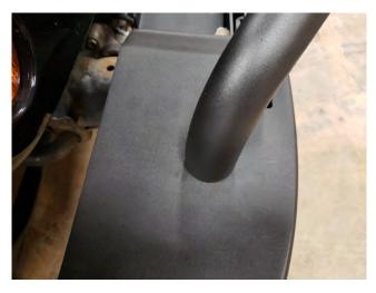
**STEP 7** // Install the optional overrider bar to the bumper using the (4) M8x1.25x25mm bolts, lock washers, and flat washers.
