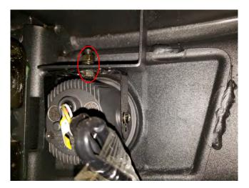
**STEP 6** // Install the (2) fog lights to the bumper using the (2) M5x0.8x15mm bolts, and lock nuts.
