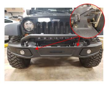
**STEP 8** // Insert the bumper through the front of the winch plate, and through the frame rail mounts. Next insert the (2) winch plate brackets. Secure the front bumper to the vehicle using the (4) M10x1.5x35mm bolts, (8) M10 lock washers, (8) M10 flat washers, and (4) M10 nuts. Torque to 40 ft-lbs.
