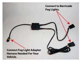
**STEP 10 // Fog Light Wiring Installation:**
