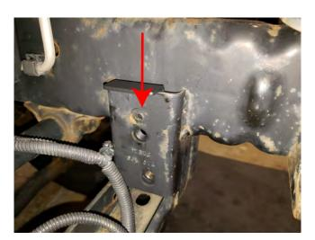
STEP 4 // Insert the (2) frame rail brackets (1) for each side into the frame rail pocket. Make sure the (2) bolt holes line up with the holes in the frame rail.
