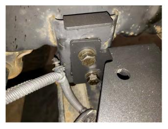
**STEP 5** // Install the winch plate to the frame rail brackets installed in the last step using the supplied (4) M12x1.75x30mm bolts, lock washers, and flat washers. Torque to 40 ft-lbs.
