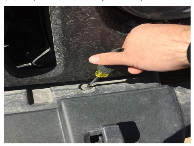
2. Remove factory plastic skid plate, there are 3 screws under the bumper, and once those are released there are 2 screws holding a vertical support that face the rear of the jeep.
