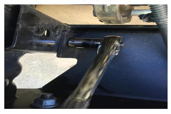
14. If installing factory tow hooks, remove the bolts you installed to hold the plate in place in step 12, having friend hold bumper, or use a floor jack or jack stand to support the bumper) and place the angled end piece on bumper, and use the tow hook to sandwich the end cap as seen below. The 4 bolts on the tow hook will fit through the mounting holes, and you will reuse the factory nuts from step 3 to tighten bracket, using the 18mm socket.
