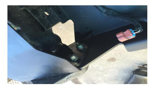
13. Install the supplied 1/2" x 1 1/2" bolt through the winch plate and through the frame as on left and right side, from inside the frame horns, and secure with the supplied flag nuts, using the 3/4" wrench or socket.
