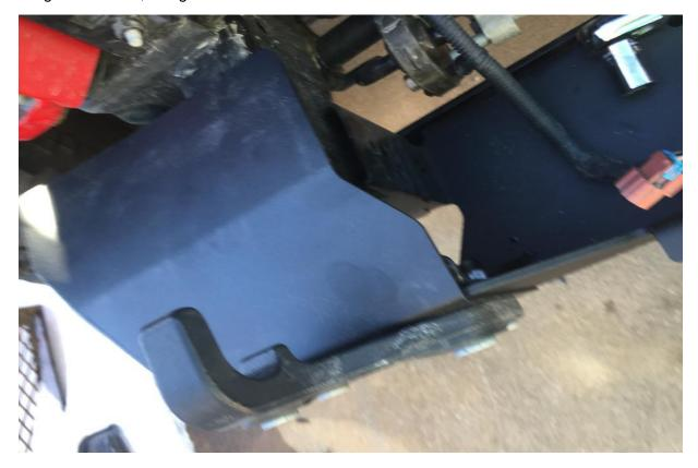
If using D ring bracket from Rough Country, or not using factory tow hooks, put end cap in place and using the supplied allen head bolts, 8mm allen wrench, washers, and nuts you can install the end cap.
