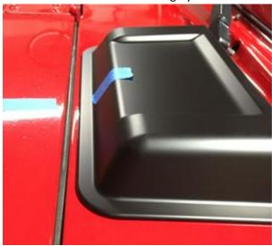
**4.** Start to peel back the protective covering on the three pieces of double sided tape. DO NOT REMOVE THEM ALL THE WAY. Just enough so it sticks out when you set the vent scoop back on the hood.
