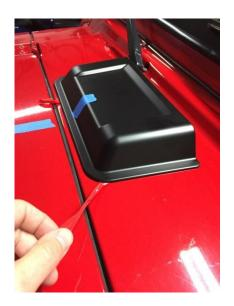
7. Remove the two pieces of masking tape used for alignment.
