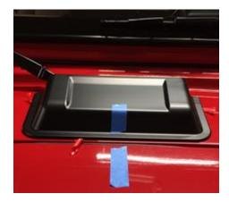
**6.** While holding the vent scoop in place, carefully peel back the protective covering from double side tape. Press down along the edges of the vent scoop to ensure good adhesion to the hood.
