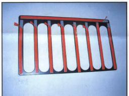
2. First, prep the area around the vent by cleaning it and then wiping it with alcohol. Then, position the Vent Cover over hood vent on vehicle. Center the slots on the Vent Cover over the slots in the vent. Ensure that the tape backing tabs are exposed. Lower the vent onto the surface of the vehicle and press down over the areas of exposed tape to hold the vent in position.
