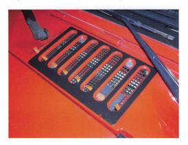
3. With the Vent Cover in position, pull the tape backing from between the tape and the body of the vehicle. Remove all tape backing in this manner. Press down around the perimeter and between all slots to ensure good adhesion of the tape.
