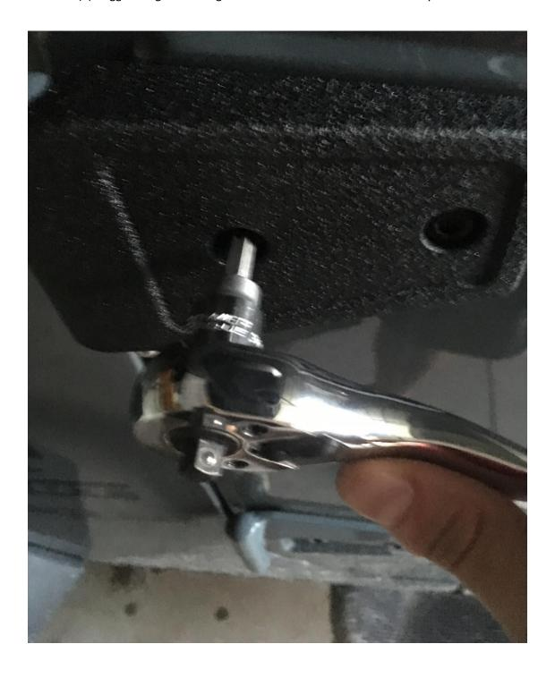
6. Replace your T-40 Star bit on your ratchet with the T-50 Star Bit again and then remove the bottom door hinge.
