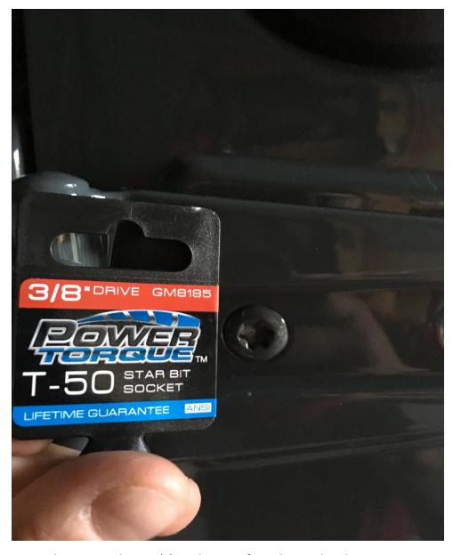
2. Using the T-50 Star bit remove the two (2) stock screws from the top door hinge.
