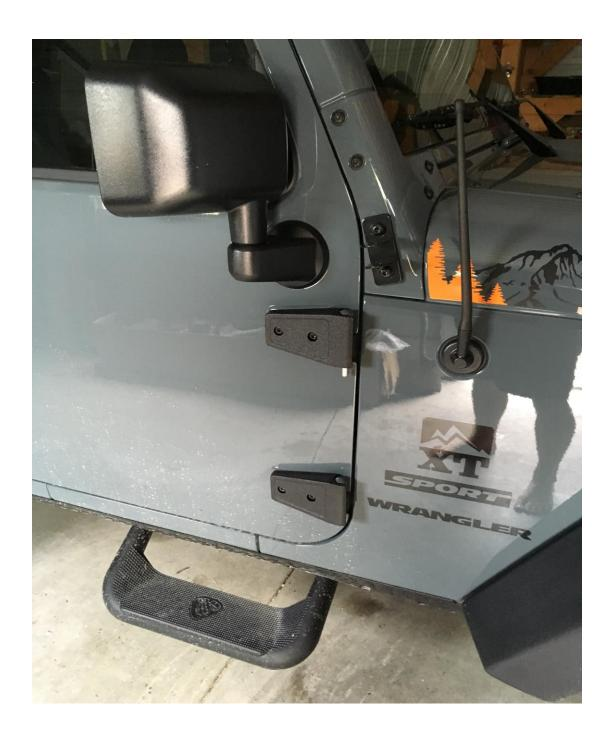
9. Repeat Steps 1-6 for your hood as well. For your hood, you can remove all of the stock screws with your T-50 Star Bit and install all of the Rugged Ridge hinge covers using your T-40 Star bit so long as your hood is locked in place.
