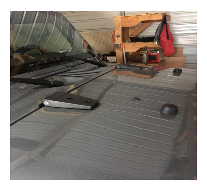
10. The new screws will come very slightly loose over the next two (2) to three (3) days so go back over all of the Rugged Ridge hinge cover screws with your T-40 Star Bit a few times over the next two(2) to three (3) days to make sure that the screws have not come loose.
