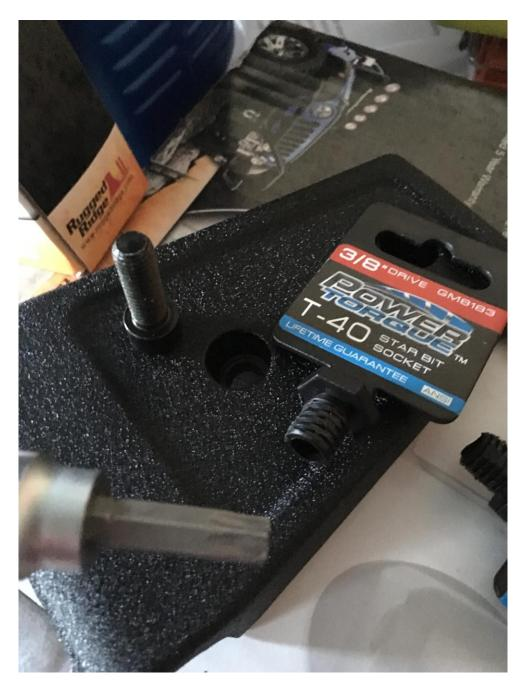
4. Take one (1) Rugged Ridge door hinge and place it flush over the stock door hinge.
