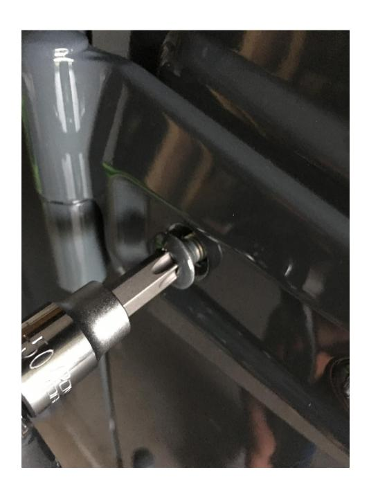
3. Replace your T-50 Star bit with the T-40 Star bit on your ratchet as the Rugged Ridge door hinges utilize the T-40 Star Bit.
