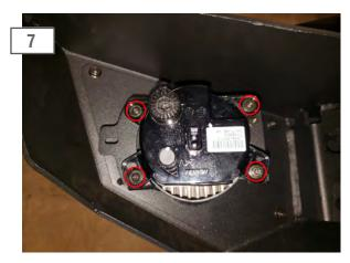
Install the factory fog lights to the fog light mounts using the (4) M4 allen bolts, washers, and nuts.
