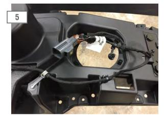
Remove the factory foglight harness from the factory bumper using a trim panel removal tool. \*\*Note, the factory bumper is two pieces. You will have to remove all (24) 7mm screws to gain access to the foglight harness.
