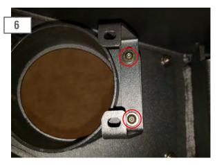
Install the (2) LED fog light brackets to the fog light mounts of the bumper using the (4) M4 allen bolts, washers, and nuts.
