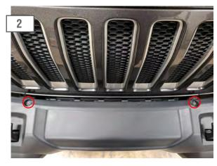
Remove the (2) upper plastic push pins securing the plastic cover to the frame rails.
