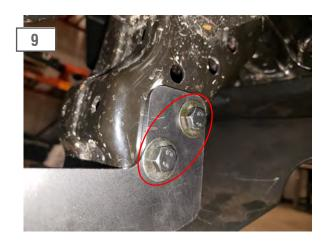
**Optional Skid Plate:** Install the skid plate brackets to the lower frame rail of the vehicle using the (2) M8 bolts, flat washers, lock washers, and nuts.
