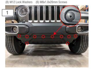
From under the vehicle, remove the (8) plastic push pins securing the factory splash shield to the vehicle. Next remove the (2) 8mm screws, and remove the splash shield from the vehicle.
