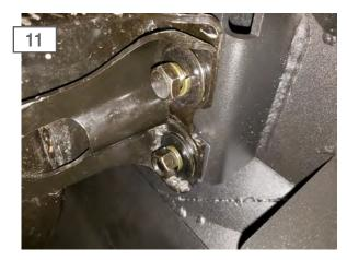
Attach the bumper to the frame using the (8) M12 nuts, lock washers, and flat washers. Torque to 40 ft-lbs.
