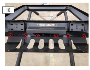
**Optional Skid Plate:**Attach the skid plate to the bumper using the (6) M6 allen bolts, lock washers, flat washers, and nuts.
