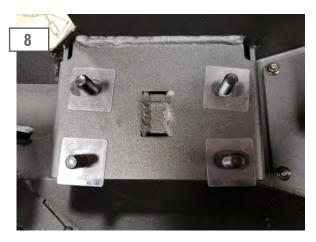
Insert the (2) dual bolt plates through the back side of the bumper mount and secure using the plastic holders.
