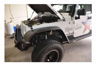
5. Remove fender flare and drill the holes just marked with a  $\frac{1}{2}$ " drill bit in order to install nutserts
