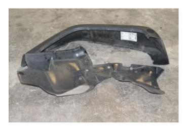
10. Hold the liner into its originally location to determine where to trim for the area of liner that will no longer fit with the new fender flare. With a marker, draw a line to trim the liner
