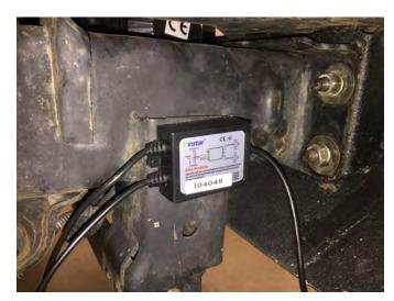
**Step 4\\**Mount the ballast to the frame using self taping screws.
