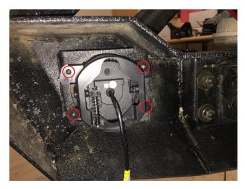
**Step 3\\**Install the new LED fog lights using the factory hardware.
