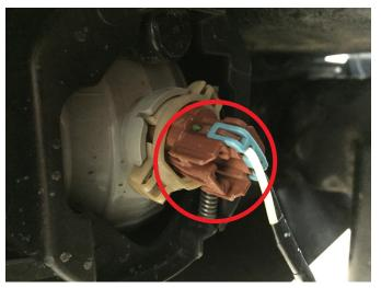
**Step 1\\**Access the connectors on the rear of the fog lights from the wheel well, and remove.
