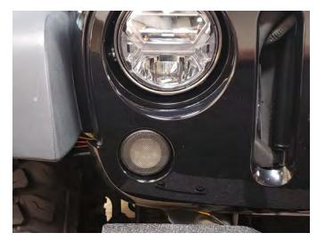
**Step 7\\**Test the lights before completion. Reinstall the grille.
