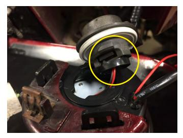
**Step 6\\**Connect the LED turn signal harness into the factory turn signal socket. Twist the socket clockwise to tighten.
