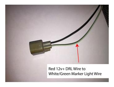
**Step 5\\**Locate the front side marker light wiring harness. Run the red 12v+ wire from the turn signal light, and splice into the white/green marker light wire.
