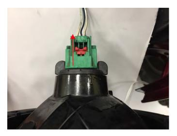
**Step 3:** Slide the red retaining clip away from the plug. Then disconnect the plug from the headlight.
