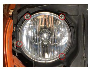
**Step 2:** Using a T15 Torx bit, remove the (4) torx screws securing the headlight to the vehicle.
