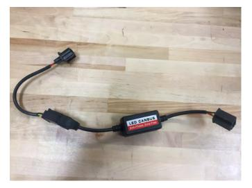
**Step 4:** Connect the adapter harness to the anti-flicker harness as shown.
