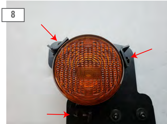
8 Insert the factory turn signal lights to the upper turn signal brackets. Once they are clipped in place, insert the (3) M6 x 20mm bolts to lock the light in place.
