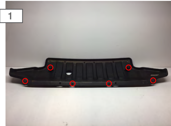
Remove the (6) plastic push pins securing the factory splash shield to the vehicle. (4) Across the front edge, (2) on the rear edge.
