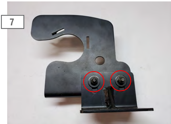
7 Install the upper and lower turn signal brackets together by using the (2) M6 x 20mm bolts, flat washers, and nuts.
