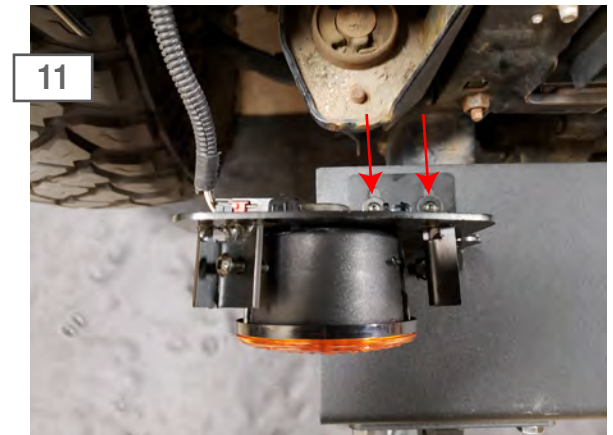
11 Plug the turn signal harness into the turn signal. Attach the turn signal bracket to the bumper using the (2) M6 x 20mm bolts, washers, and nuts.
