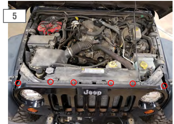
Locate, and remove the (6) push pins holding the grille in place. Gently pry the lower part of the grille away from the vehicle, unplug the turn signal lights, and remove the grille completely.
