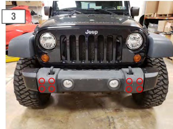
From under the vehicle, access and remove the (8) 18mm nuts securing the factory bumper to the vehicle.
