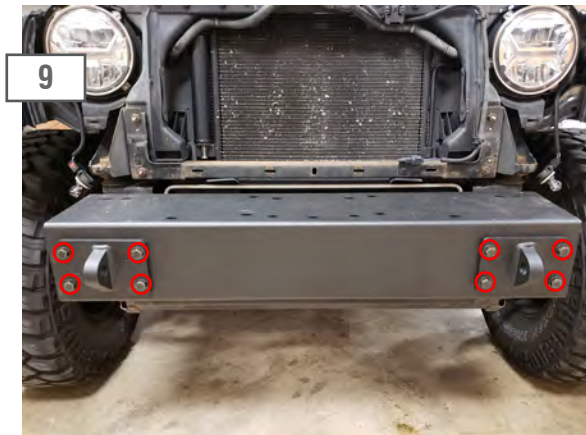
9 Install the D-Ring brackets to the bumper, and then to the frame of the vehicle using (8) M12 bolts, (16) flat washers, (8) lock washers, and (8) nuts. Torque to 40 ft-lbs.
