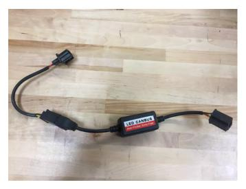
**Step 5:** Connect the adapter harness to the anti-flicker harness as shown.
