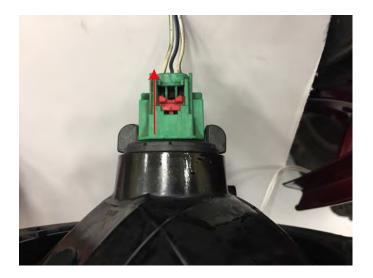
**Step 3:** Slide the red retaining clip away from the plug. Then disconnect the plug from the headlight.
