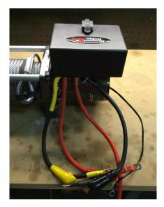
7. Remove the nut and washer on the post with red paint. Install the red wire on this post. Tighten the nut with a 14mm wrench, and feel free to use another wrench on the back side of the post to prevent it from turning while you tighten the nut.
