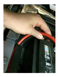
19. Using a 10mm socket/ratchet or wrench, use the provided accessory post to mount your wires. Attach the red wire to the positive battery terminal. Attach the black wire to the negative battery terminal.
