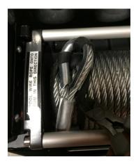
22. Move the cable down past the winch frame and through the fairlead hole in your bumper.
