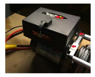
6. Turn the winch around on your workbench. Untangle and straighten the wires from the solenoid box to make it easy to install them onto the winch. Slide the rubber protective sheaths down each wire.
