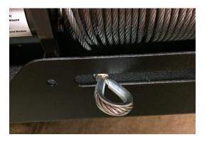
23. Attach the fairlead to the bumper using the 2 stubby bolts and nuts, using an 18mm socket/ratchet and an 18mm wrench. Depending on the location of the cable hole in your bumper, use the appropriate mounting holes in the fairlead. Once mounted, slide the cable through the fairlead.
