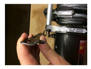
4. Use the supplied allen wrench along with one of the supplied screws to finish mounting the bracket. Tighten both screws to securely fasten the bracket.
