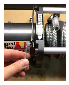
5. Slide the solenoid box into the bracket. Using the supplied allen wrench, tighten both screws on the solenoid box.
