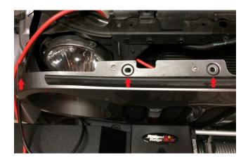
14. OPTIONAL: I chose to wrap part of the red wire with black electrical tape. It offers additional protection, as well as hides the red wire from being visible from the front of the vehicle. Only wrap the portion of the wire visible from the grill area.
