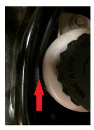
17. Continue routing your wires under the plastic piece just to the left of the battery.
