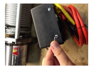
3. Using the 6mm allen wrench, remove the screw from the rear post on the top of the winch. Place the bracket on the left-hand side of the winch, reinserting the screw you just removed. Don't fully tighten.
