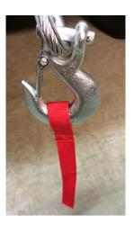
28. Attach the latch to one of the steel rings on your bumper, then use the remote control to gently tighten the cable. In this picture, I placed the cable below the right fairlead roller to keep it from rubbing on the steel roller itself during travel (note that I did <u>NOT</u> place any noticeable load on the cable after attaching; this location is to prevent rubbing and for aesthetics). This step is entirely optional and feel free to place the cable in the location of your choosing.
