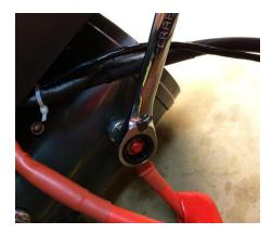
8. Slide up the rubber protective sheath so that it covers the post completely. Repeat step 7 and 8 for the short yellow and short black wires.
