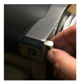
12. Insert the 4 longer bolts into the underside of your bumper and into the bolt holes of your winch. The bolts will screw into the square nuts you just inserted. From under your bumper, tighten with the 5/8" socket, ratchet and extension.
