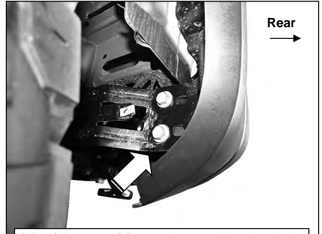
(Fig 2) Remove (2) outer bumper bracket bolts
