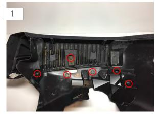
Begin by removing the factory fender liners, there are (5) 10mm bolts. Remove the factory marker light harness from the light and zip tie it out of the way. Remove the factory fender by firmly pulling it away from the vehicle. Start from the front of the fender and work towards the rear. The factory clips will most likely break, the clips will not be reused.
