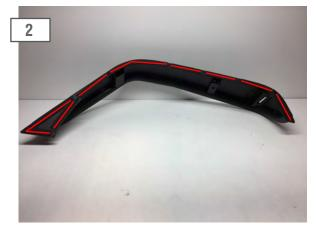
Install the supplied foam on the back side of the fenders as seen above.
