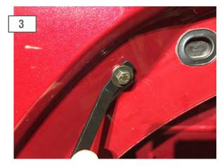
Using the supplied handle and long M6x1.0 install the rivnuts. Hold the rivnut in place with the handle and tighten the rivnut securing it to the vehicle.
