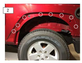
Install the supplied rivnuts in the (8) holes circled above. Begin by drilling the rivnut holes to 23/64".
