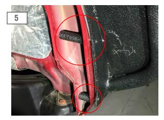
Install the supplied spacers between the inner and outer fenders using the M8x1.25 120mm bolt for the long spacer and the M8x1.25 65mm bolt for the shorter spacer.
