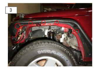
Install the Barricade Flat Fenders using the supplied M8x1.25 25mm long Allen bolts, install the forward most (5) bolts first. \*\*Note: Loosely install all hardware before fully tightening bolts to ensure proper bolt hole alignment.
