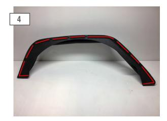
Install the supplied foam to the fender before installation.
