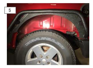
Install the M6x1.00 25mm bolts with the supplied washer and lock washer on all locations with the installed rivnuts.
