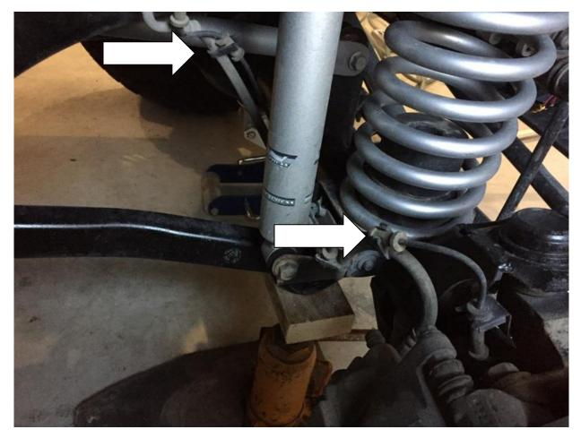
4. Secure the new brake line bracket to the frame using the factory bolt with the 10mm socket.
