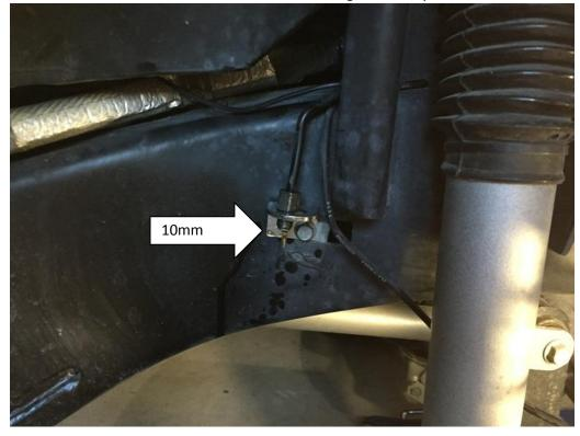
5. Place the new brake line through the hole of the bracket and secure it with the spring clip. Attach the steel brake line to the new flexible brake line. Leave nut slightly loose to allow adjustment of brake line.
