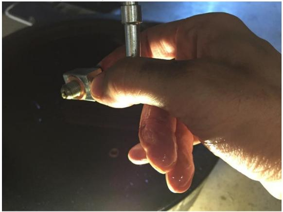
7. Rotate brake line so that it is out of the way of any other objects. Torque down caliper bolt and finish tighten down steel brake line using the 12mm and 17mm wrench.
