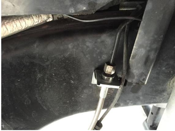
6. Remove brake line from caliper using the 15mm socket. Reuse factory bolt to secure new brake line to caliper. You will need to place one crush washer, brake line, than another crush washer. Secure to caliper with elbow of new brake line facing the rear using 15mm socket.
