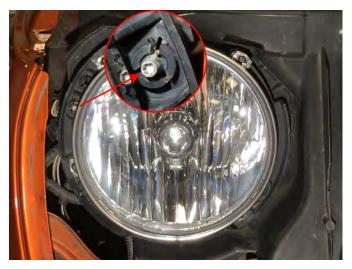
**Step 6:** Headlight Adjustment: Using a T15 torx bit, turn the adjuster clockwise to adjust the light up. Turn the adjuster counter-clockwise to adjust the light down.
