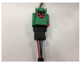
**Step 5:**Connect the factory headlight harness into the supplied headlight harness connectors, and then into the back of the LED headlight. Push in the red clip to lock harness in place.
