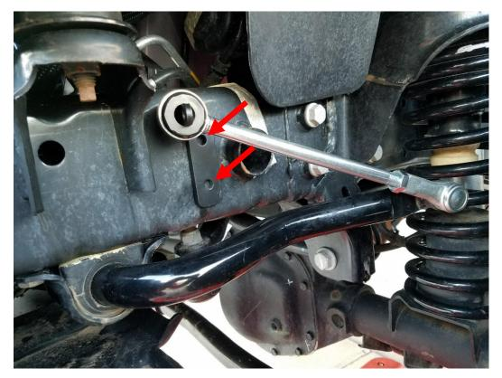
**9.** Using the supplied self-tapping bolts with a ½" socket, install the mount bracket. I found it easiest to use an impact wrench to get the bolts started. But then, use a normal wrench to fully tighten so that you do not strip them.
