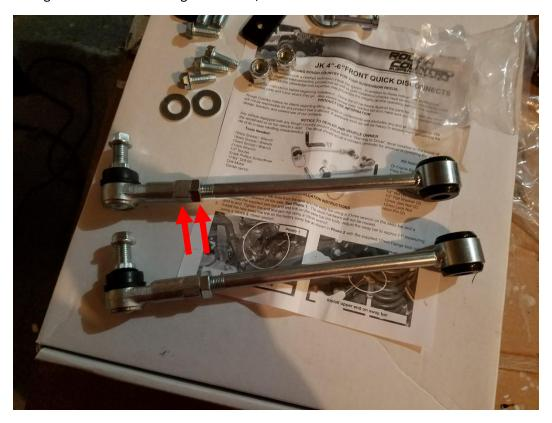
**5.** Using a 15mm socket and 14mm wrench, attach the upper end link to the sway bar on the driver side. Torque to 75ft/lbs.
