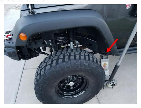
**3.** Rotate the sway bar down so give you easy access to the top of the sway bar link. Using an 18mm socket and 19mm wrench, remove the sway bar link.
