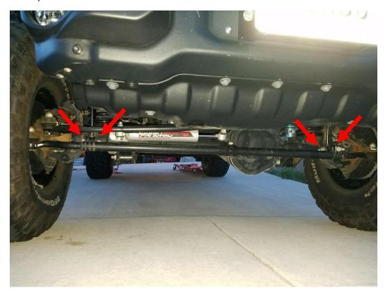
2. (Recommended, Not Required) Use a jack and jack stands to lift the driver side frame of the jeep. This will give you a lot more room to work with. You can also remove the wheel, or turn the wheel to give you even more room. I chose to leave the wheel on.
